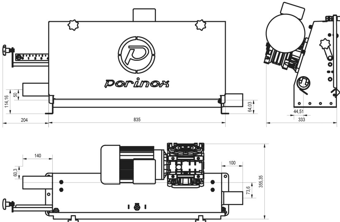
The Drag Unit of Porinox is an **automatic system** driven by a **1,5kW** motor-reducer, which distributes the animal feed through a chain system.
